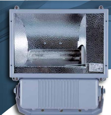
High performance premium quality floodlight with precision optics incorporating either a 250 or 400 watt metal halide or high pressure sodium discharge lamp.
